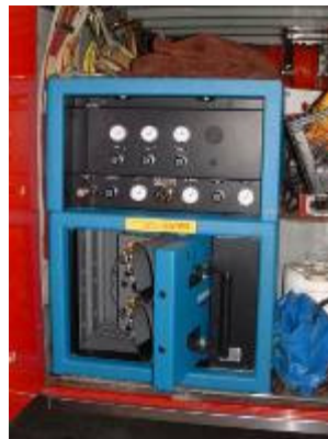
Eagle Air SideWinder X2 Containment design fill enclosure offers operator protection in the event of SCBA cylinder or component rupture. This two-position fill station offers a compact, space saving design allowing for mounting in small compartments.
